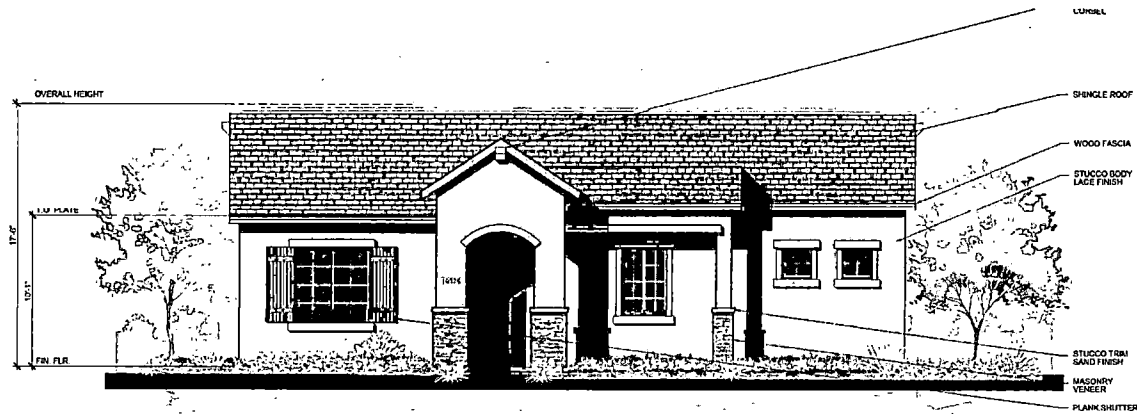
Front Elevation Elevation A 1/4" = 1'-0"
